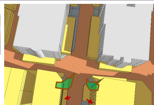
Activate chamfer-sides by provision of openings (windows, doors), entrance for people or landscaped gardens
